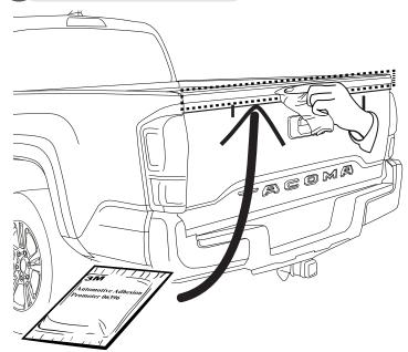
A full surface contact between tape and substrate is decisive for good adhesion performance. Contact is achieved by applying pressure. In practice a pressure between 40 and 50 N/cm² is usually needed and an application temperature between 25 and 45 °C or 77 and 113 °F is also necessary. During application, add-on parts and tapes must have the similar temperature.
