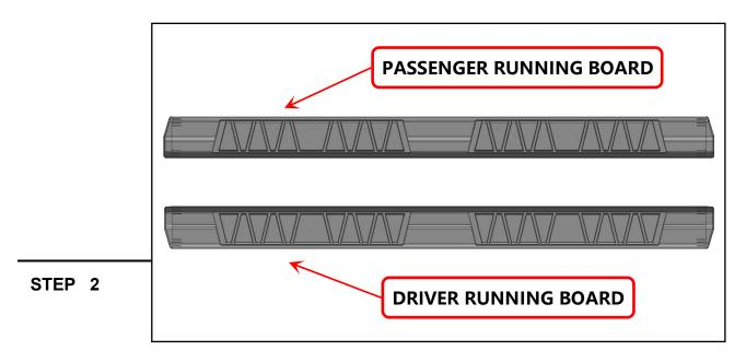
Identify each side step by the front of the Running Board. Notice: "D" for Driver/Left Side; "P" for Passenger/Right Side.
