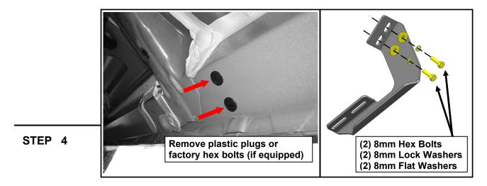
Remove the plastic plugs or hex bolts. Loosely fit the (1) Driver Center/Rear step bracket to the vehicle threaded body hole using (2) M8 x 30mm bolts, (2) M8 lock washers, and (2) M8 flat washers. Do not fully tighten to allow for later adjustments. Repeat this step for all Driver Center/Rear step brackets.
