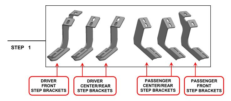
Please identify each mounting bracket using the engraved location identifier. Notice: The center bracket and rear bracket are interchangeable.
