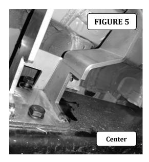
**Step-3** Position the frame mount slider bracket up to the frame rail, align and hook the upper hole in the center and rear brackets with the bolts previously installed into the frame. Secure in the bottom holes of the center and rear brackets using (2) M10 x 25mm Hex bolts, (2) M10 flat washer, (2) M10 lock washer, (FIGURE 5). Leave the bolts loose for final adjustment.
