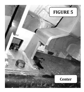
**Step-3** Position the frame slider bracket up to the frame rail, align and hook the upper hole in the center and rear brackets with the bolts previously installed into the frame. Secure in the bottom holes of the center and rear brackets using (2) M10 x 25mm Hex bolts, (2) M10 flat washer, (2) M10 lock washer, (FIGURE 5). Leave the bolts loose for final adjustment.
