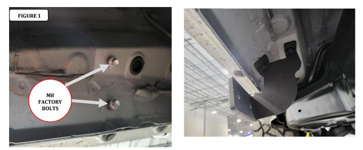
**Step-3** Locate the (2) M8 factory bolts in the underside of the body panel, at the center of the cab (FIGURE 3).
