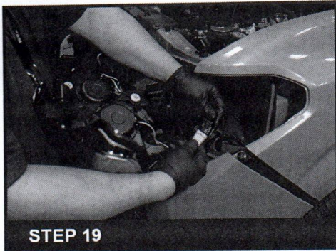
STEP 19 Reconnect the headlight harness
