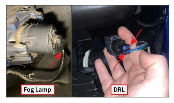
Route the LED lighting wiring towards the RH side headlight and fog light assembly. Splice the LED lighting harness into the vehicle following the diagram below.
