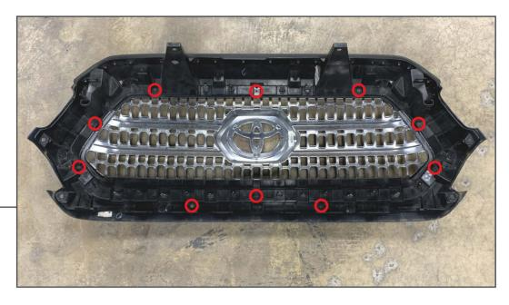
Remove (10) Phillips screws from the back-side of the grille.
