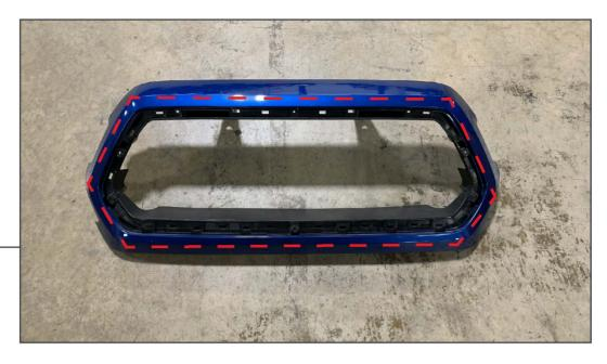
Using exterior detailer and a microfiber cloth, clean the inside edges of the grille housing.
