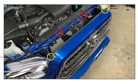
Open the vehicle hood. Remove (2) 10mm bolts and (2) plastic push clips from the vehicle grille.
