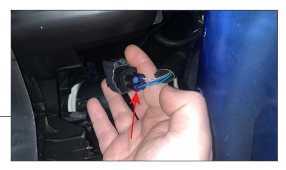
Route the LED lighting wiring towards the RH side headlight assembly. Splice the LED lighting harness into the vehicle DRL harness following the diagram below. The lights will power on with the DRL.
