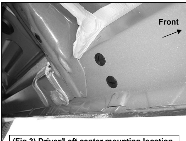
(Fig 3) Driver/Left center mounting location
