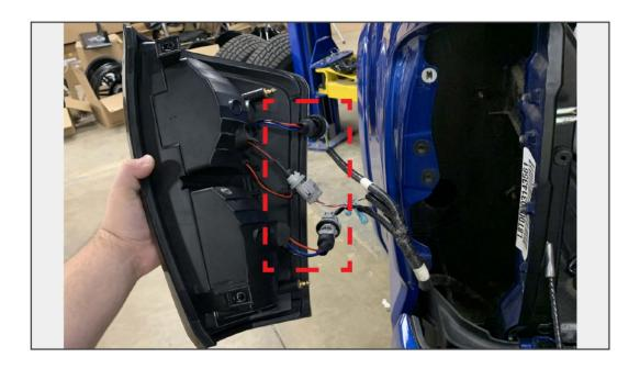
The LED tail lights are sensitive to polarity. If the polarity is incorrect, the tail lights will not function correctly.
