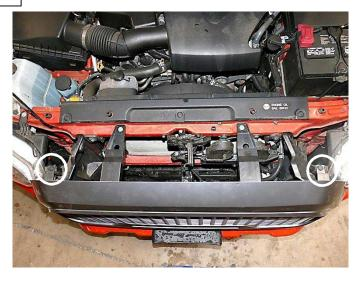
Step 2 Reinstall 2 factory clips circled above to secure grille in place.
