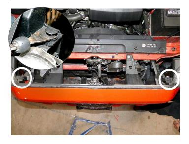
Step 1 Open vehicle's hood. Using a plastic removal tool or similar tool locate and remove 2 factory clips circled above holding the factory grille onto vehicle. Save hardware for reinstallation.
