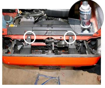
Step 2 Using a 10mm socket locate and remove 2 factory bolts securing the factory grille onto vehicle. Save hardware for reinstallation.
