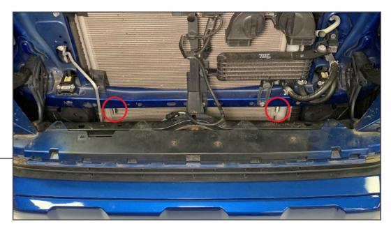
Locate the holes along the bottom of the lower cross bar on the vehicle. Insert (2) M10 stud plates into the (2) holes along the bottom.
