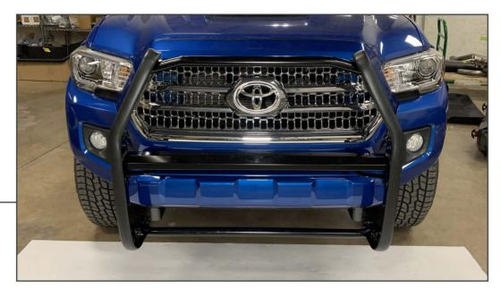
Fully tighten the mounting brackets secured to the vehicle in steps 4-6. Re-install the grille to the vehicle using the original hardware.
