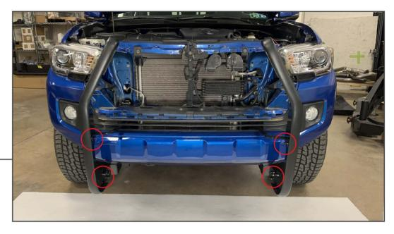
Loosely install the LH and RH push bars to the mounting brackets using (8) M10 x 35mm bolts, (16) M10 flat washers, (8) M10 lock washers, and (8) M10 nuts.
