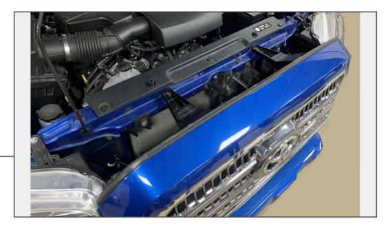
Open the vehicle hood. Remove (2) 10mm screws and (2) plastic push clips from the vehicle grille assembly. Once the hardware is removed, lift the grille brackets over the screw holes and remove the grille from the vehicle.
