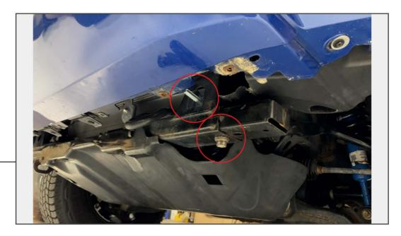
Behind the bumper, locate the vehicle frame. Install (1) M10 stud plate into the hole in the frame, and hold into place using (1) M10 plastic stud retainer. Loosen and remove (1) 17mm bolt.
