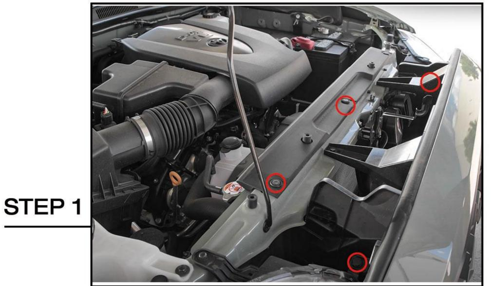
Use tools to remove two bolts and two clips.
