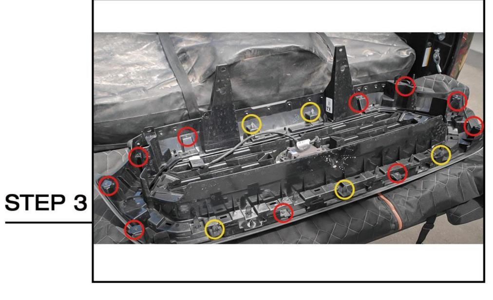
Remove all screws and clips around the original grille and take out the original grille.
