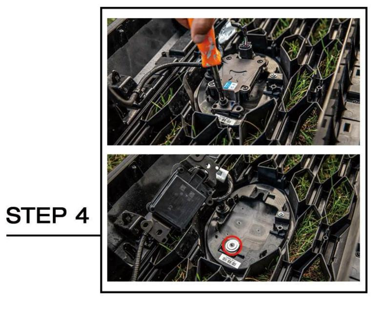
Remove Tss sensor. If you don't have a TSS sensor, you can skip this step. The bolts that were unscrewed with the screwdriver sit in a circular nut you see above. These nuts, along with the screws, need to be reused in your new grille.
