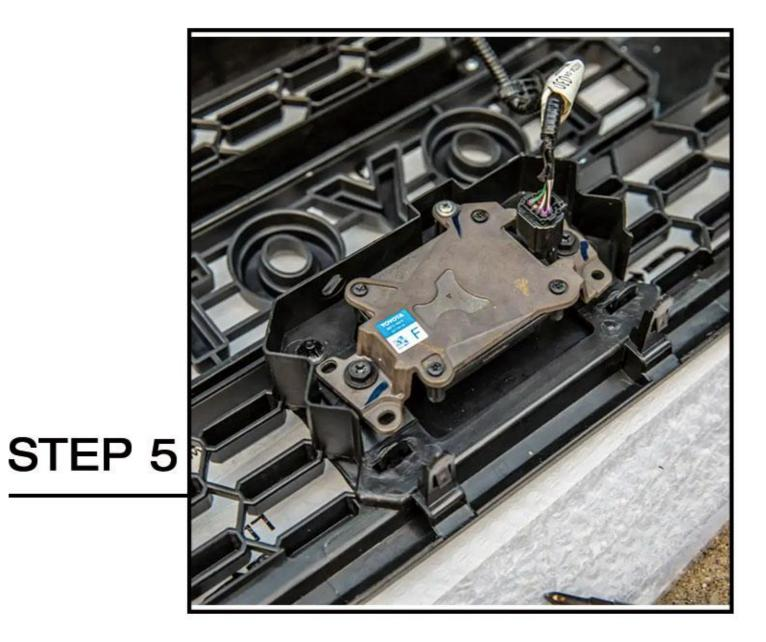
Transolant TSS Sensor into new grille. Install the circular nuts you removed in the last step. There is an identical channel in the garnish you prepped earlier. Place the TSS in the orientation seen above, and tighten down the 2 bolts that attach it to the grille.
