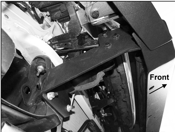
(Fig 14) Passenger/right side of Bumper attached to Mounting Bracket
