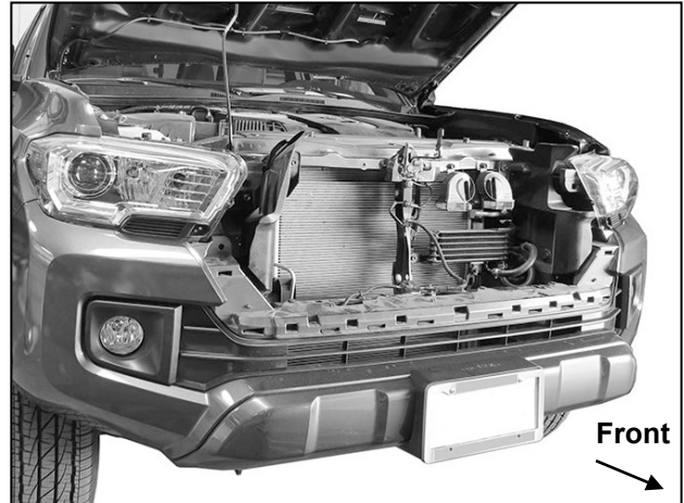
(Fig 2) Remove grille, air dam from below bumper and license plate.
