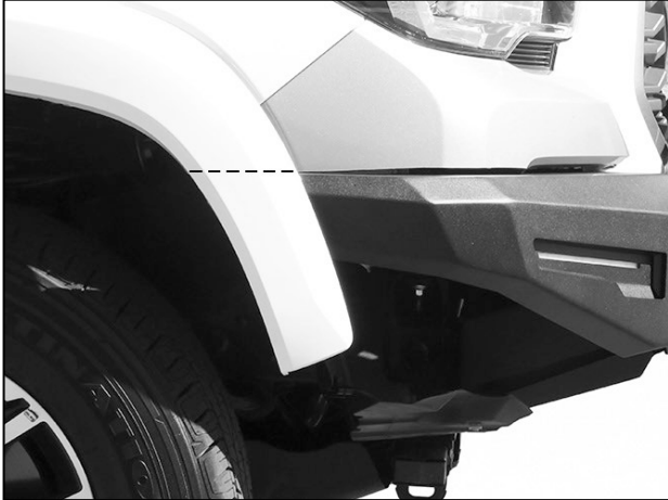
(Fig 18) Draw a straight line on fender flare to match Bumper. Use a hacksaw blade or knife to cut leading end off of fender flare
