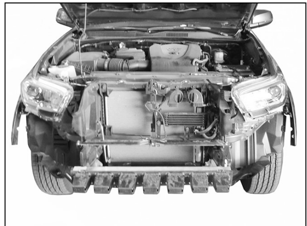
(Fig 4) Remove plastic impact bumper and aluminum crossbar and bumper brackets
