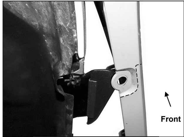
(Fig 19) Cut fender flare around mounting point if possible
