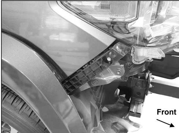
(Fig 3) Pull ends of cover off of inner clips to release and remove plastic bumper cover
