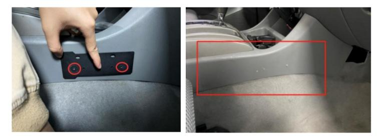
**Step 2:** Use a 1/8" drill bit to drill 2 holes into center console. Install Part "A" & "B" with Part "H" & "C".
