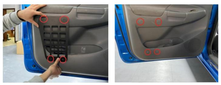
**Step 2:** Use a 1/8 " drill bit to drill the 4 holes into the plastic. Install the Part "A" with the Part "H".
