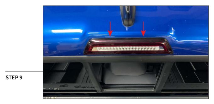
Place the LED third brake light into the vehicle, ensure the (2) metal tabs secure into the vehicle. Follow steps 1-4 in reverse order to re-assemble the vehicle.
