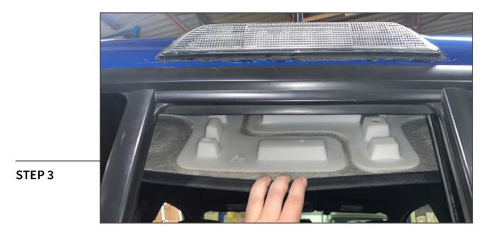
Open the rear sliding window on the vehicle. Locate the headliner board and push downwards to reveal the vehicle roof.
