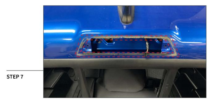
Using isopropyl alcohol and a microfiber cloth, clean the vehicle of any remaining gasket material.
