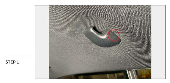
From inside the vehicle, remove the plastic cover from the rear hook using a flat head screwdriver at the designated cutout.
