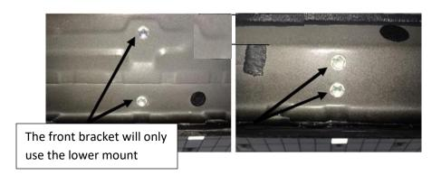
**Step 3:** Starting with the driver side, position step up to the body of the vehicle and align the brackets up with the factory mounting locations.
