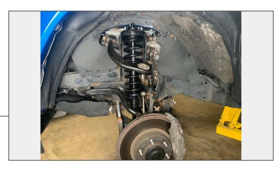
Re-assemble the vehicle suspension following steps 1-8 in reverse order using original hardware.
