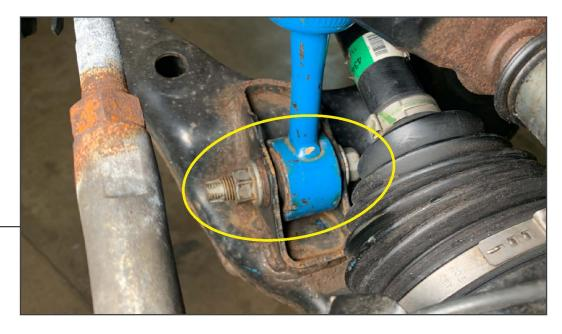
Remove (1) 21mm bolt from the bottom of the strut assembly.
