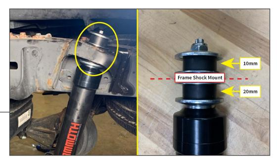
Install the top of the shock absorber to the frame mount using the provided hardware and bushings.
