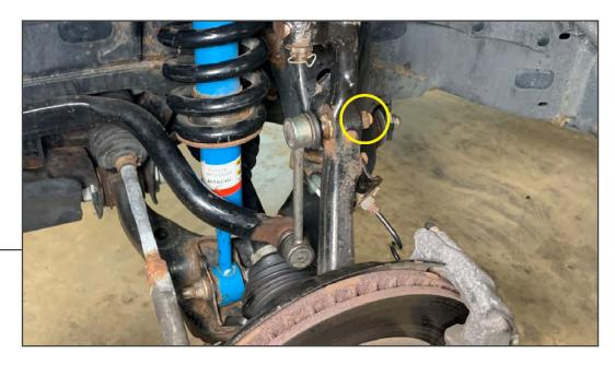
Remove (1) 17mm nut from the top of the sway bar link. \*\*It is suggested to remove the sway bar link on the opposite side at this time to allow the sway bar to move away from the strut assembly.
