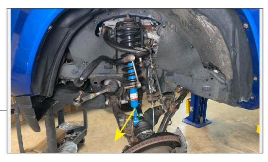
Rotate the sway bar assembly towards the front of the vehicle, then support the bar in place away from the strut assembly. Lower the strut assembly from the vehicle.
