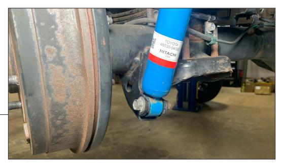
Remove (1) 17mm bolt from the bottom of the shock absorber. Remove the shock absorber from the vehicle.
