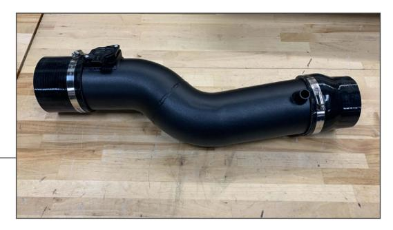
Prepare the intake pipe for installation. Install (1) 4" - 4" coupler on the side closest to the MAF sensor. Install (1) 3" - 4" coupler towards the PCV hose port. Slide (2) 4" hose clamps over each coupler.
