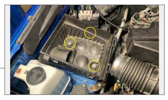
Remove (3) 12mm bolts from the air box base. Remove the air box base from the vehicle.
