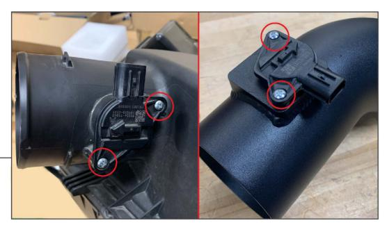
Remove (2) Phillips screws to remove the MAF sensor from the original air box. Transfer the MAF sensor to the new intake tube using the provided hardware. Do not over tighten.
