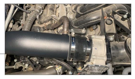
Install the vehicle PCV hose to the intake pipe. Secure to the intake pipe re-using the original spring clamp.
