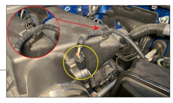
Open the hood of the vehicle. Firmly pull up to dislodge the engine cover, then pull the cover off the hinge. Un-plug the MAF sensor from the air box. Using a flathead screwdriver, gently pry the plastic retainer upwards to release the wiring harness from the air box lid.
