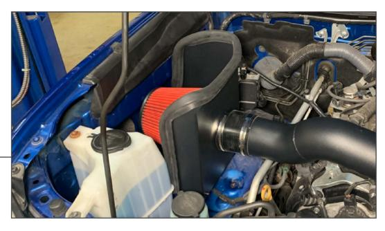
While holding the air filter to the heat shield, align the intake pipe to the air filter. Secure the air filter to the intake pipe by tightening the previously installed hose clamp.
