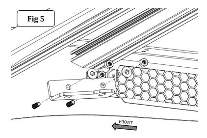
**Step-6** Install (1)  $\frac{1}{4}$ " x 1" button head screws with  $\frac{1}{4}$ " plastic washer in the central hole of the side rail. Place the center bracket onto the side rail, align the screws with the hole in the center bracket. Secure the center bracket using (1)  $\frac{1}{4}$ " lock washer, (1)  $\frac{1}{4}$ " flat washer and (1)  $\frac{1}{4}$ " hex nut. Snug but do not tighten the screw, (Fig 6).
