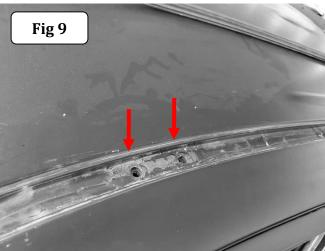
**Step-10** Place the spacers on the roof rail over the factory nuts (Fig 10). Lay the trim next to the roof rail where it was removed and mark the area the spacers ocuppied.
