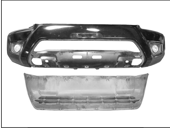
(Fig 10) Lower cover removed
