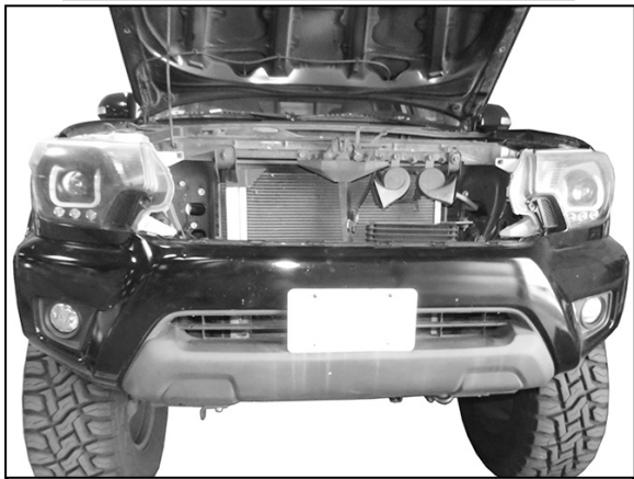
(Fig 3) Remove cover and grille. Remove hardware attaching top of bumper cover to remove cover
