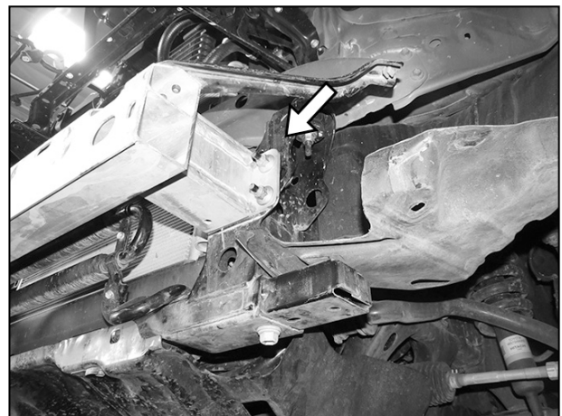
(Fig 4) Remove the (2) outer hex nuts from the driver/left aluminum impact bumper bracket. NOTE: Pictured with plastic bumper cover removed for instruction purposes only, it is not necessary to remove bumper cover
