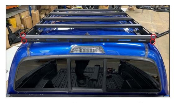
Install the rear cross bar inside the side rails using (4) M8x1.25 x 25mm Allen bolts, (4) M8 lock washers, (8) M8 flat washers, and (4) M8 nuts. Tighten hardware until secure.
