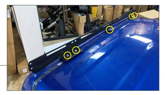
Install (1) side rail to the vehicle using (5) M6x1.00 x 50mm bolts, (5) M6 lock washers, and (5) M6 flat washers, and (5) M6 spacers. Place the spacers against the vehicle, then align the side rail to the spacers and install the provided hardware. Do not tighten until all hardware is threaded into the vehicle.
