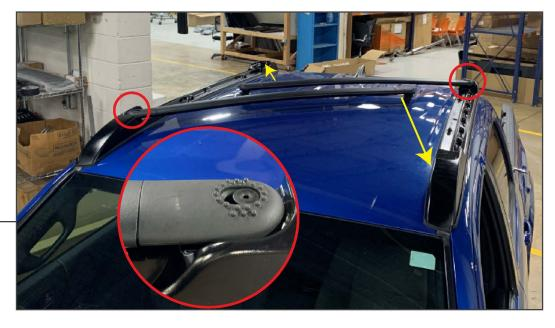
Swing out both roof rack bars towards the opposite side of the vehicle. Place down until the arms clip into place. Tighten down the (1) Allen bolt on each roof rack bar.
