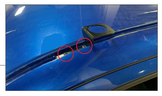
Using the front bolt holes, secure the roof bracket to the vehicle using (2)  $M6x1.00 \times 16mm$  Allen bolts.
