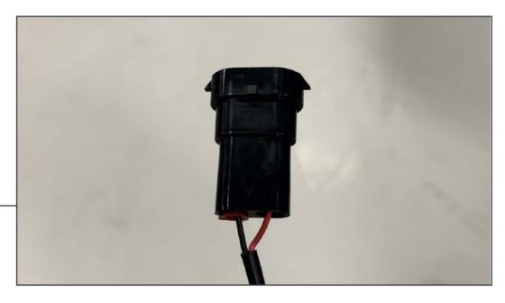
Using the appropriate fog light connector and DRL module, insert the (2) wires into the connector following the below diagram. Take note on which way the connector installs to ensure proper wire lead installation. Ensure the wire leads click into the connector and the gaskets are seated.
