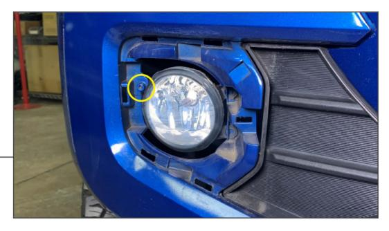
Remove the (1) Phillips screw from behind the fog light to release the fog light from the bumper.
