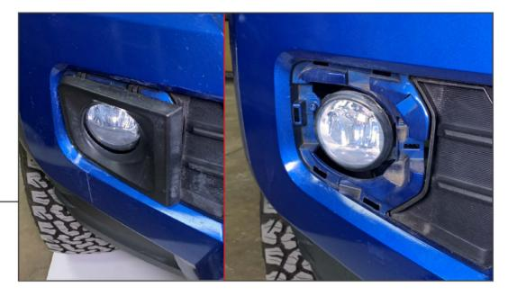
Remove the fog light outer bezel from the front bumper. Use a plastic panel removal tool to release the clips securing the bezel to the bumper.
