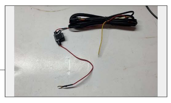
Splice the DRL harness into the vehicle's wiring following the diagram below.
