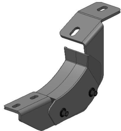
(Fig 4) Push center pin in to expand Clip in Bracket
