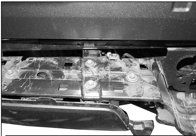
(Fig 3) Models with receiver hitch, remove the hex bolts attaching bumper to top of hitch
