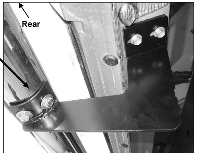
(Fig 4) Driver side rear mounting location pictured
