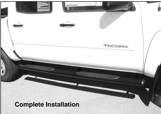
(Fig 3) Driver side center mounting location pictured
