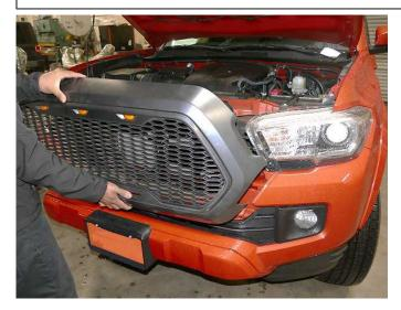
Step 1 Place supplied grille (A) onto vehicle as shown above.
