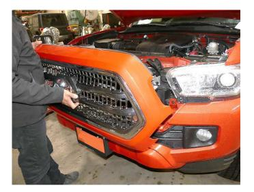
Step 3 Firmly grab and pull factory grille off of vehicle. Discard factory grille.
