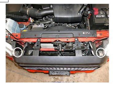
Step 2 Reinstall 2 factory clips circled above to secure grille in place.
