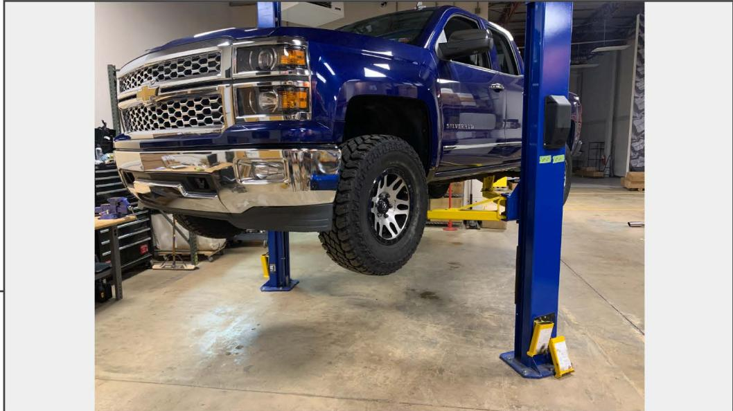
Raise the vehicle so that the tires are just off the ground. Support the vehicle with jack stands.
