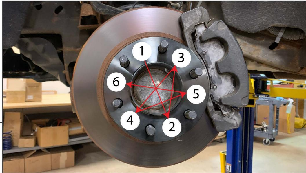
Install the wheel spacer using the supplied lug nuts. Tighten all lug nuts by hand in a star pattern. Then, torque the lug nuts as follows for your application: Tacoma: 83ft.lbs.
