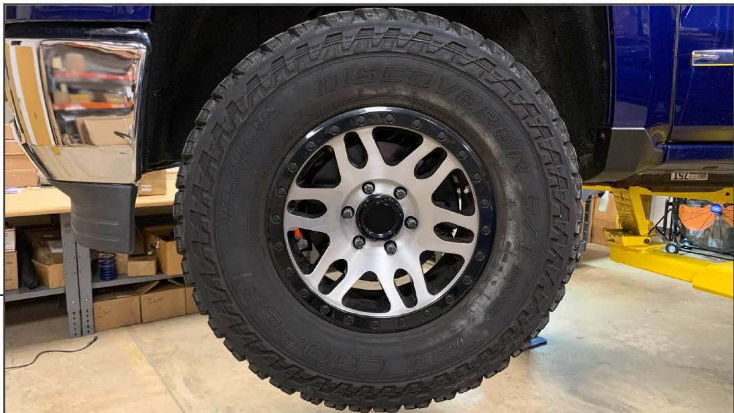
Using a lug wrench, remove the wheel.
