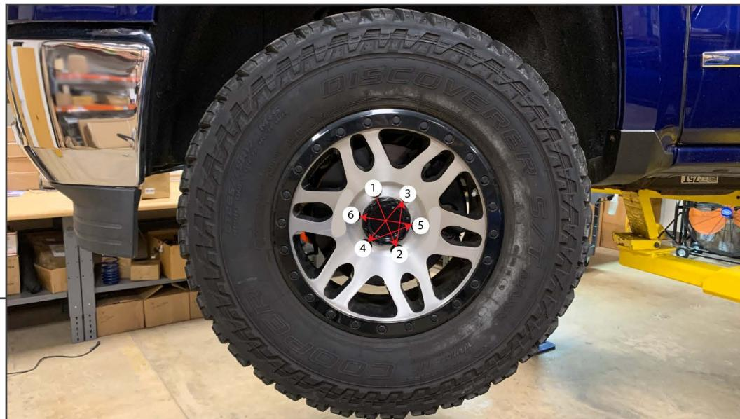
Reinstall the original wheel on the new studs. Then, torque the lug nuts as follows for your application: Tacoma: 83ft.lbs.
