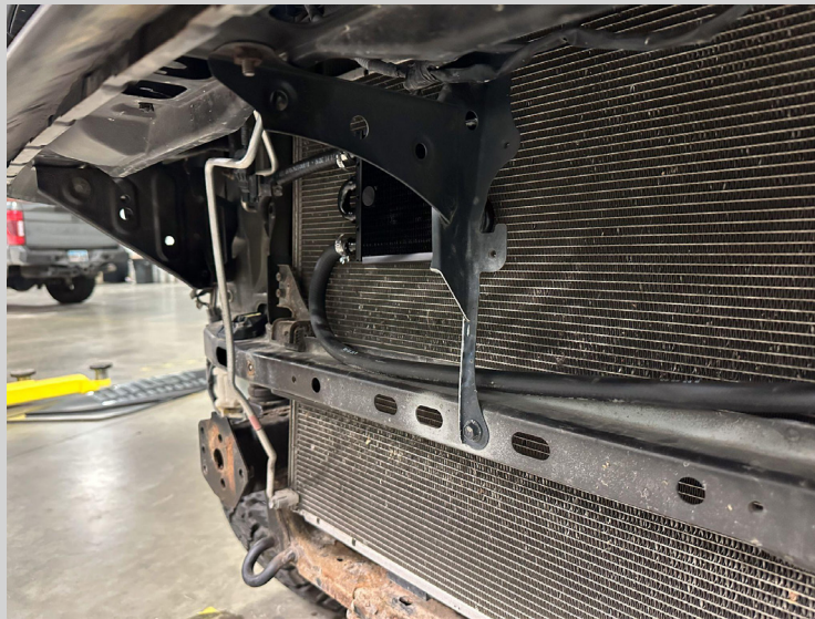
Figure 4: Center brace trimmed for winch.
