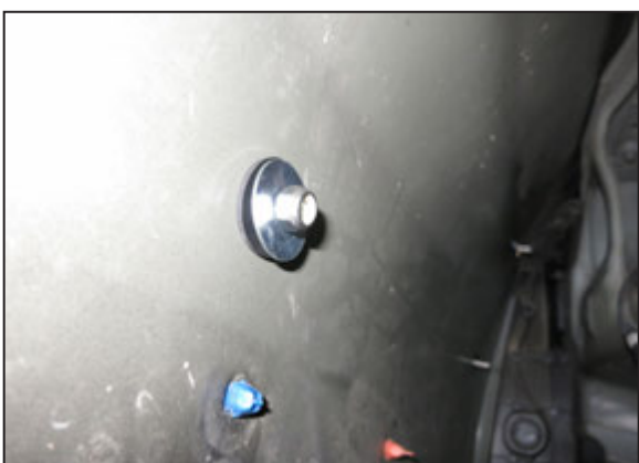
23. Secure the snorkel to the fender using the nuts and fender washers provided.
