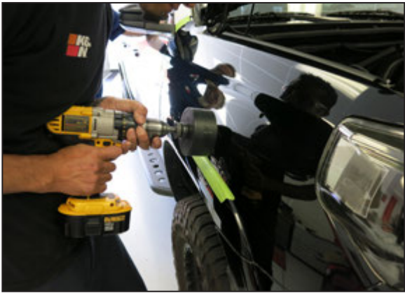
15. Drill the hole for the snorkel outlet with a 4-1/4" hole saw. Deburr the hole.
