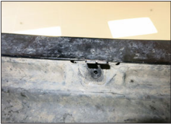
26. Reinstall the inner fender and secure with the factory hardware. NOTE: Replacement black screw grommets are provided incase the factory grommets break.
