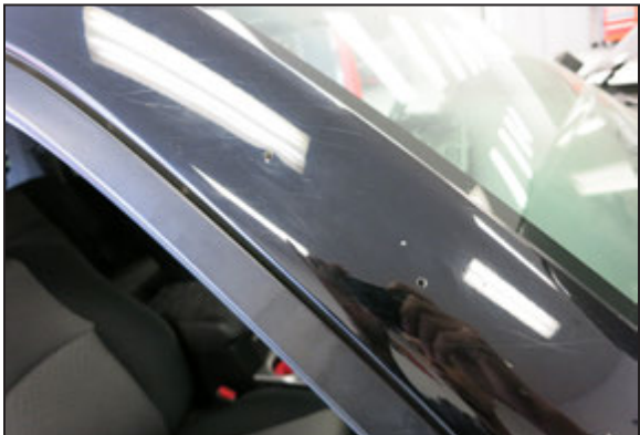
19. Use a 3/16" drill for the "A" pillar mounting bracket holes. Go slow and do not push hard while drilling to prevent drill bit wander or walk. Use tape or vacuum hose to create a 5/8" stop on the drill bit so the drill will only go 5/8" past the outer sheet metal.
