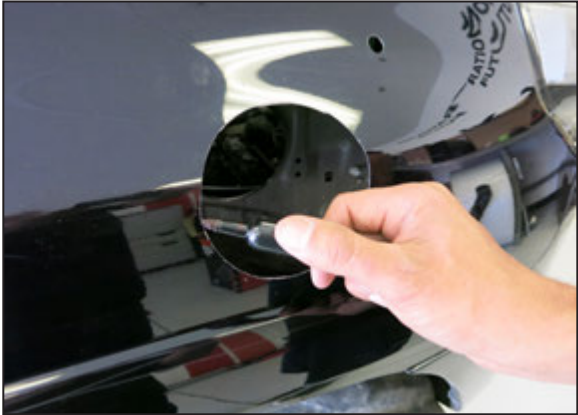
16. Use touch up paint or similar paint to paint the raw metal to prevent corrosion.
