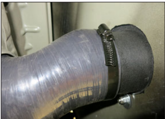
25. Install the coupling hose through the hole in the inner fender and connect it to the snorkel outlet. Secure with the provided hose clamp.
