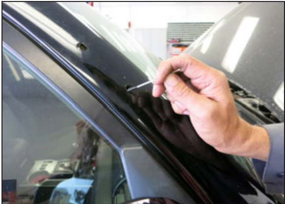
20. Use touch up paint to paint the raw sheet metal to prevent corrosion.
