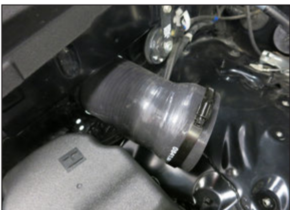
24. Secure the snorkel to the "A" pillar bracket with the hardware provided.
