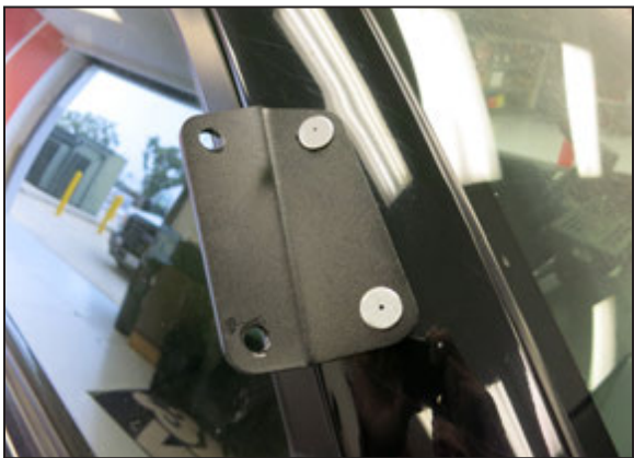
21. Install the snorkel bracket onto the "A" pillar using the provided rivets.
