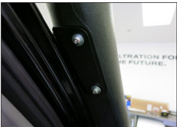
24. Secure the snorkel to the "A" pillar bracket with the hardware provided.
