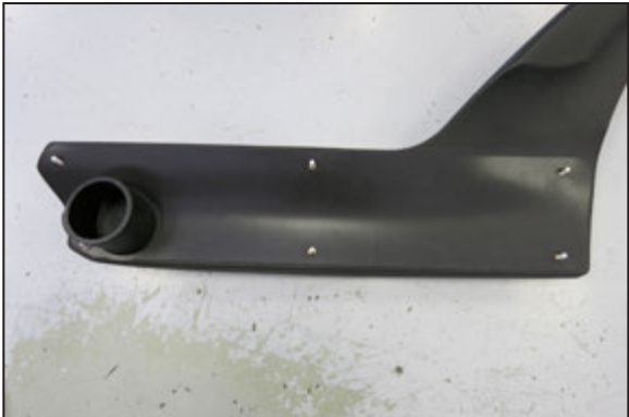
17. Apply threadlock to the M8 Studs and screw into the inserts on snorkel and leave the studs out 3/4". Apply gasket material to the back of the snorkel.
