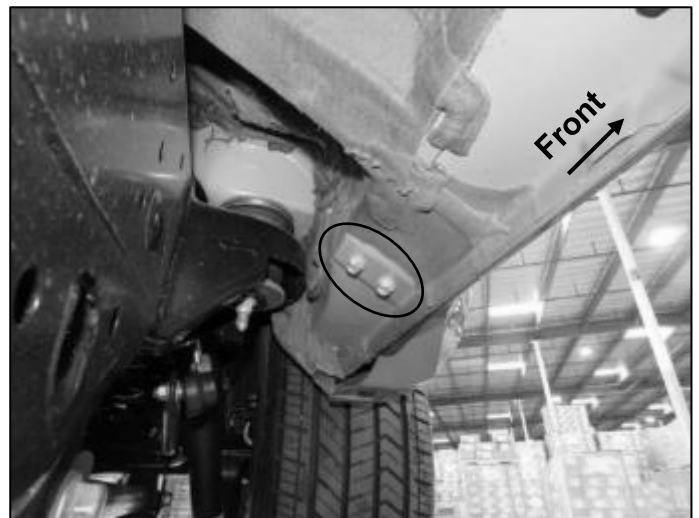
(Fig 4) Locate the rear mounting points circled and remove the OEM 8mm bolts.
