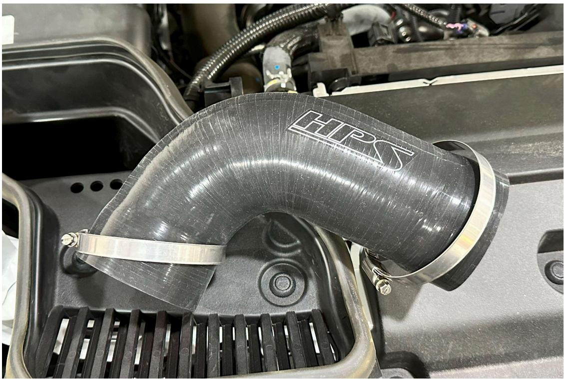
4. Place the provided embossed clamps onto the HPS silicone intake tube in the orientation shown.
