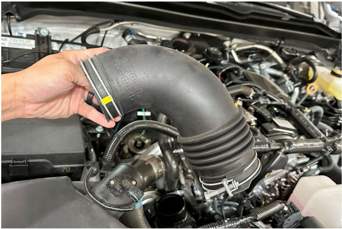
3. Disconnect and remove the stock intake tube.
