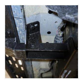
Attach the supporting bracket to the passenger's side front mounting point, using **B35** bolt, **W22** lock washer and **W23** washer, with the **N15** nut.
