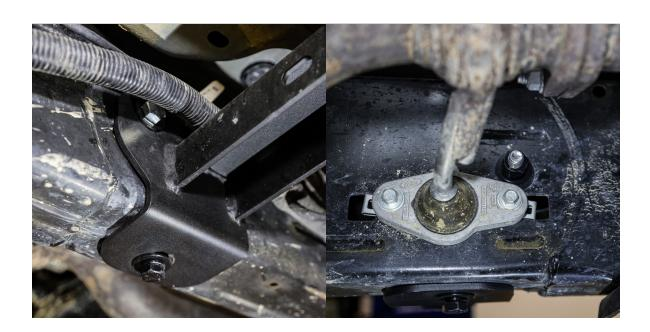
For the driver's side middle mounting point, use **B58** bolt and **W27** washer as shown to the top left. Use the **W27** washer with **W25** lock washer and **N19** nut as shown to the top right. (Do not use the oversized washer for this mounting point.)
