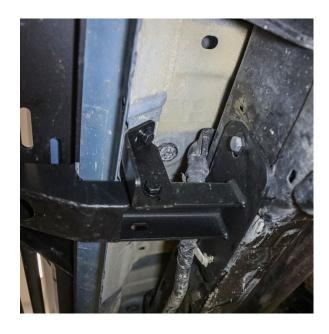
Attach the supporting bracket to the driver's side rear mounting point, using **B35** bolt, **W22** lock washer and **W23** washer, with the **N15** nut.
