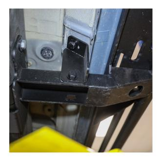
Attach the supporting bracket to the passenger's side rear mounting point, using **B35** bolt, **W22** lock washer and **W23** washer, with the **N15** nut.
