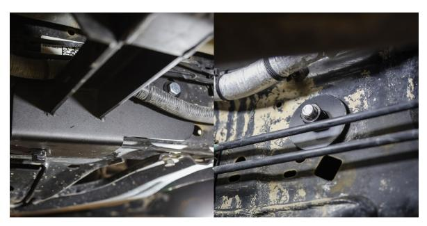
For the driver's side front mounting point, use **B58** bolt and **W27** washer as shown to the top left. Use the oversized washer with **W25** lock washer and **N19** nut as shown to the top right.
