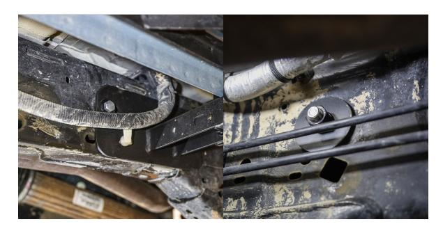
For the driver's side rear mounting point, use **B58** bolt and **W27** washer as shown to the top left. Use the oversized washer with **W25** lock washer and **N19** nut as shown to the top right.
