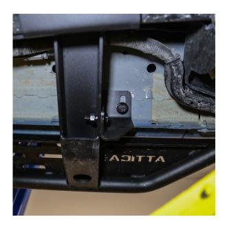
Attach the supporting bracket to the driver's side front mounting point, using **B35** bolt, **W22** lock washer and **W23** washer, with the **N15** nut.
