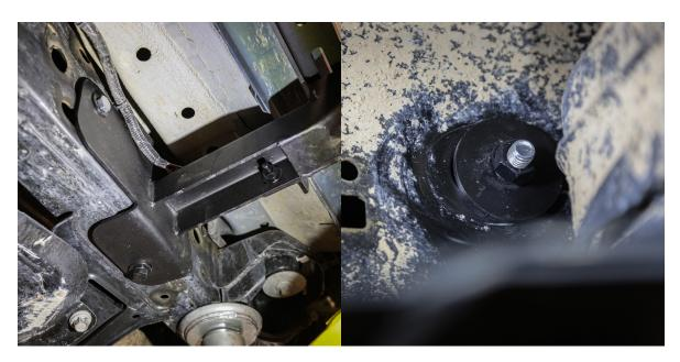
For the passengers side front mounting point, use **B58** bolt and **W27** washer as shown to the top left. Use the oversized washer with **W25** lock washer and **N19** nut as shown to the top right.
