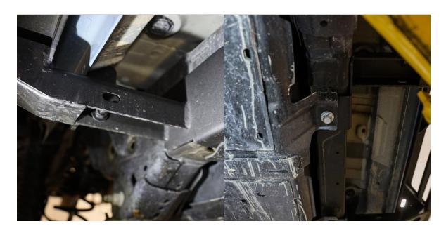
For the passengers side rear mounting point, use **B58** bolt and **W27** washer as shown to the top left. Use the oversized washer with **W25** lock washer and **N19** nut as shown to the top right.
