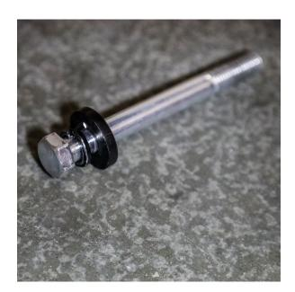
To prevent damaging your gas tank, use the supplied **W25** lock washer with the thicker washer for the passenger's side middle mounting point.
