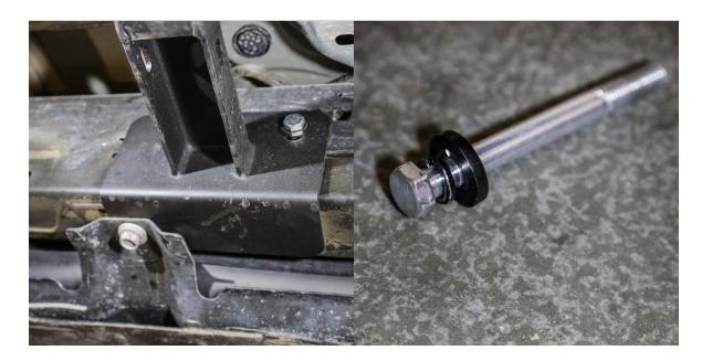
For the passenger's side middle mounting point, use **B58** bolt and the thick washer with **W25** lock washer as shown to the top right. Use the oversized washer with **W25** lock washer and **N19** nut to mount to the frame.
