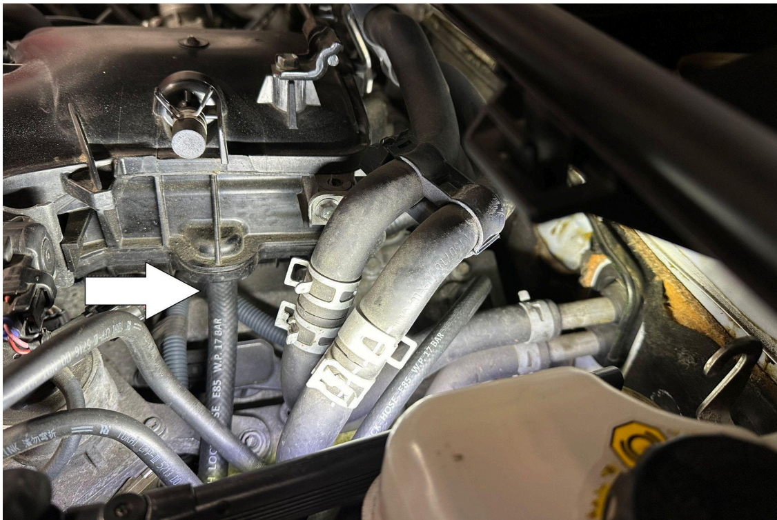
12. Install the opposite end of the assembled -6 push-on hose onto the intake manifold barb.
