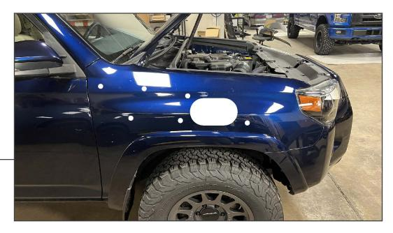
With the fender drilled, remove the template and masking tape.
