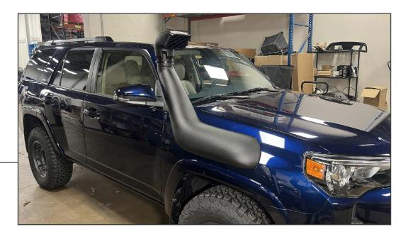
Secure the snorkel to the fender using (6) M8 flat washers and (6) M8 lock nuts. Then, secure the top of the snorkel to the A-Pillar bracket using (2) M6 combo hex bolts. Secure the snorkel top hat to the snorkel tube using (1) small hose clamp.
