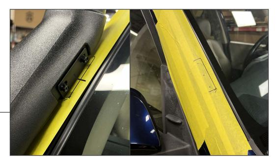
Mount the upper mounting bracket to the snorkel tube using (2) M6 combo bolts. Then, trace the mounting area of the bracket to the previously placed masking tape. Remove the snorkel tube from the vehicle. Remove the bracket from the snorkel tube.
