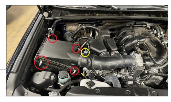
Open the vehicle hood. Loosen (1) hose clamp securing the air box lid to the intake tube. Un-clip the (4) air box lid clamps. Unplug the MAF sensor and use a pry tool to dislodge the wiring harness retainers along the air box lid.
