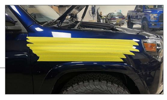
Lay out and identify all components. Using masking tape, apply tape to the fender surface to prepare for drilling.
