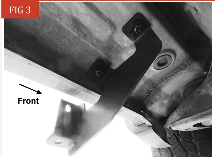
(Fig 3) Example of Driver/Left Front Mounting Bracket attached to the front location
