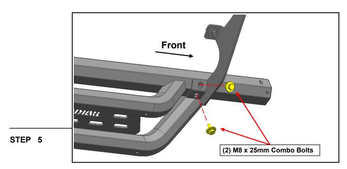
With all brackets loosely mounted to the vehicle, fit the drop step onto the brackets, and loosely secure into place using (6) M8 x 25mm combo bolts.
