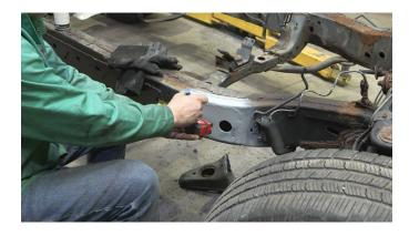
Tack weld the part on fully before fully welding it onto the frame. Following proper welding procedures, begin welding the part. 100% weld around all edges.
