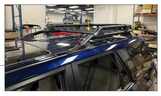
With assistance, lift the roof rack assembly onto the vehicle roof.
