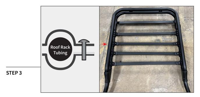
Using the (4) cross bars, (8) cross bar clamps [top], (8) cross bar clamps [bottom], (8) M6 x 40mm bolts, and (8) M6 flat washers, secure the crossbars in the desired location.
