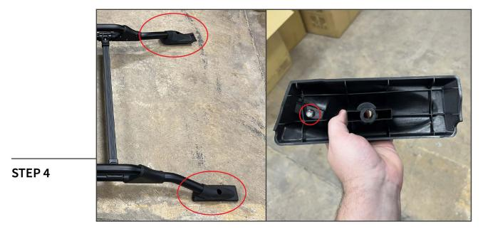
Install the front mounting brackets to the roof rack tubing. Slide the bracket onto the tubing, and remove the rubber bottom. Then, secure the bracket to the tubing through the bottom of the bracket using (1) M6 x 30mm bolt.
