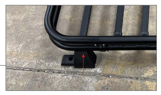
Install the rear mounting brackets to the roof rack tubing. Fit the bracket under the rear of the roof rack. Secure the bracket to the roof rack tubing threaded insert using (1) M6 x 15mm bolt and (1) M6 flat washer.
