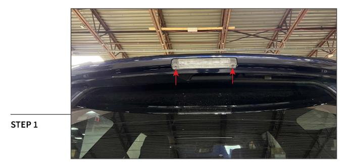
Locate the vehicle third brake light in the tailgate. Remove (2) Phillips head bolts from the bottom of the light assembly.
