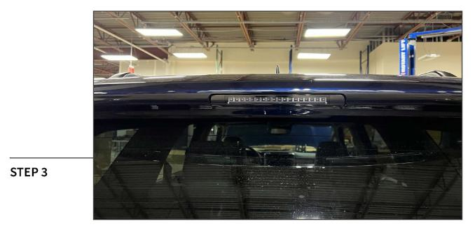
Plug the vehicle wiring harness into the new third brake light assembly until the connector locks into place. Then, re-install the third brake light into the vehicle tailgate using the original (2) Phillips head bolts. Tighten the hardware until the brake light is fully secure.
