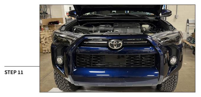
Re-install the vehicle headlights, then with the front bumper following steps 1-7 in reverse order.
