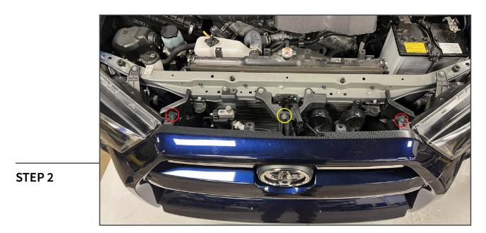
Remove (2) plastic push clips and (1) 10mm bolt from the grille assembly portion of the bumper.
