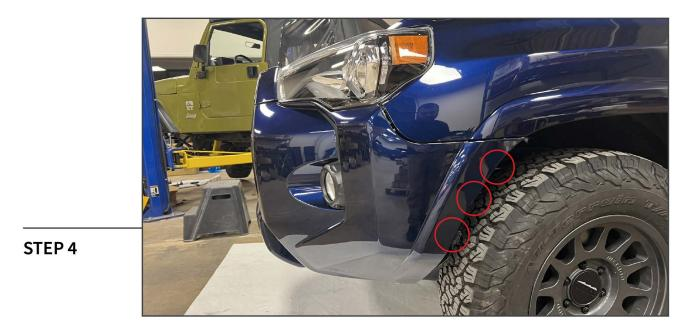
Remove (3) 10mm screws from the outer edge of the front bumper on each side of the vehicle.
