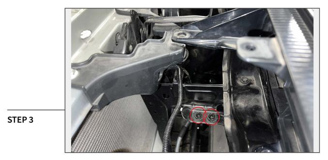
From behind the grille, remove (2) 10mm screws and unplug the Adaptive Cruise Control module, if equipped.
