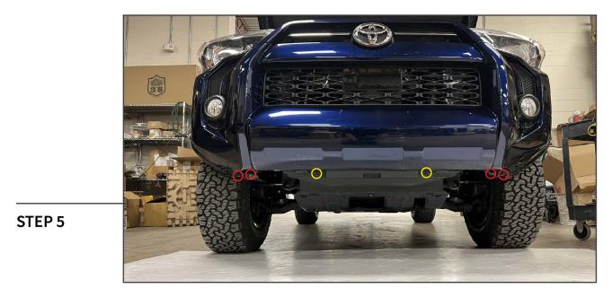
Remove (4) 10mm screws and (2) 10mm bolts from under the vehicle bumper.
