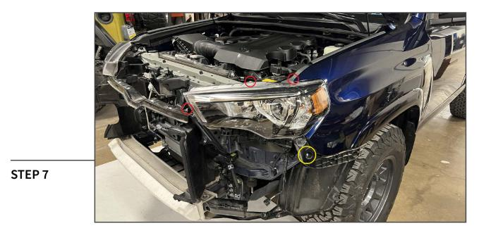
Remove (3) 10mm screws and (1) 10mm bolt from the headlight assembly.
