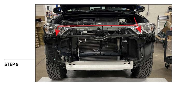
Route the DRL harness from the vehicle fuse box to each headlight mounting point.
