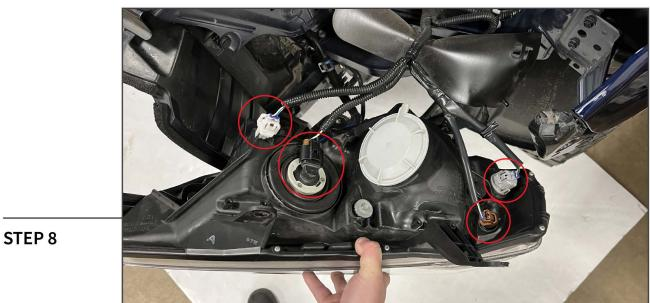
Unplug the headlight wiring harnesses. Set the original headlight aside.
