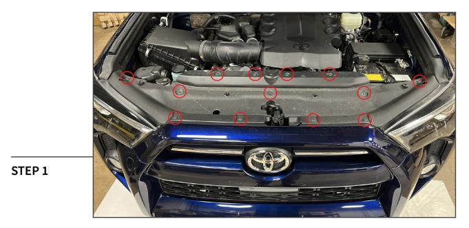
Open the vehicle hood. Locate the (13) plastic push clips. Use a panel removal tool to press the center of the clip downwards, then pry the entire clip from the radiator cover. Lift and set the radiator cover aside.
