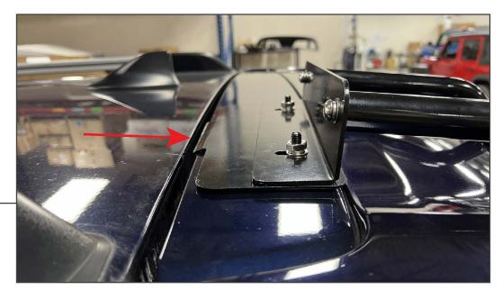
Using the hook portion of the ladder assembly, fit the hook around the top of the vehicle liftgate in the desired mounting position.
