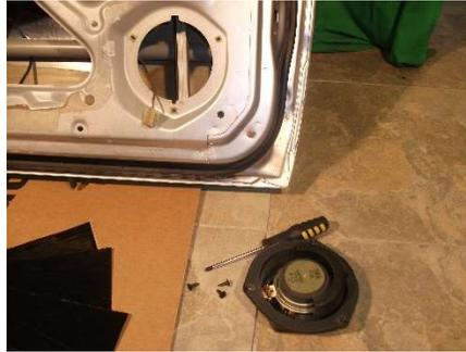
Step 2: Peel brown release paper on one sheet of HushMat Ultra (Part #10110) and apply over speaker opening as shown. Trim out center of sheet exposing the mounting hole.
