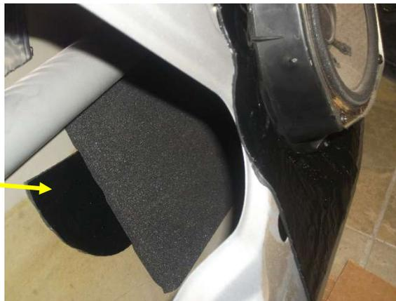
Step 4: Peel back release paper from back of one Wave Breaker pad (Part #82450) and stick the wave breaker directly on top of the round Ultra cut out you placed on the outer door skin.
