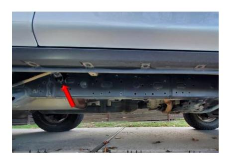
**Step 2.** Position the slider onto the vehicle frame and begin loosely installing the supplied hardware. Be sure to reattach the parking brake bracket. Once all the hardware is installed go ahead and tighten the bolts down.
