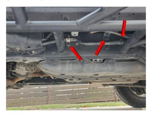
**Step 4.** Remove the 3 12mm bolts holding the gas tank skid plate
