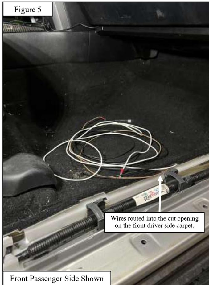
4. Route the brown door trigger wire to the passenger side B-Pillar, and the white door trigger wire under the front passenger side carpet, the center console, the front driver side carpet, and to the driver side B-Pillar.
